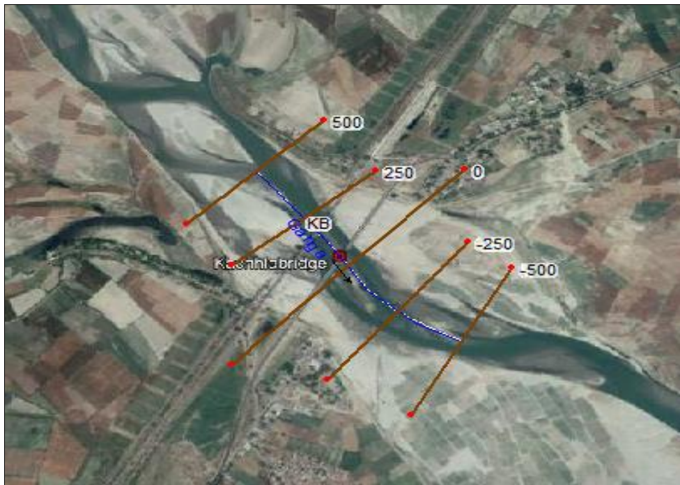
Fig. 6 : HEC-RAS Model Set up at Kachhlabridge
